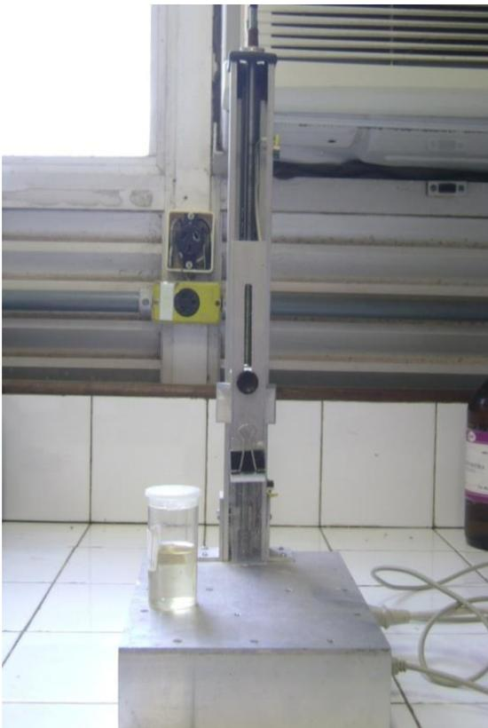
**Figura 4.7a: Máquina de dip coating**
