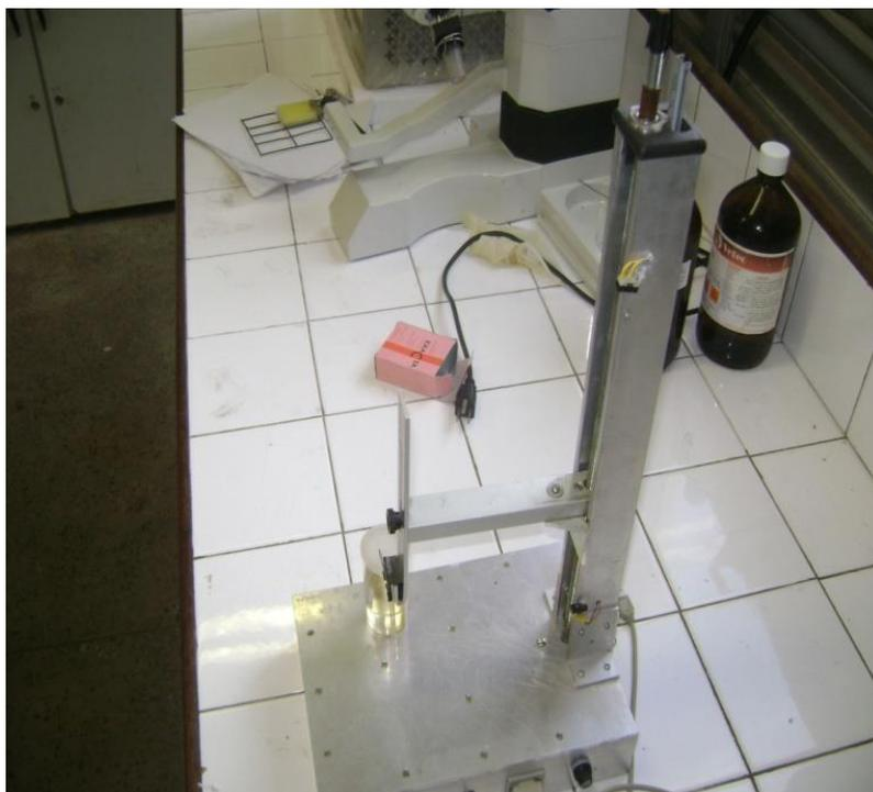
**Figura 4.7b: Máquina de dip coating.**
